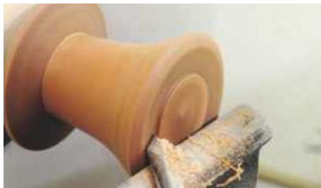
▲ Pic.8 Cut the end-grain with the gouge, so the bevel is in contact with the wood. Slow the feed speed of the tool towards the centre
